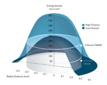
Automatic Fluence Level Adjustment Ideal balance between the total number of laser pulses and energy delivered
